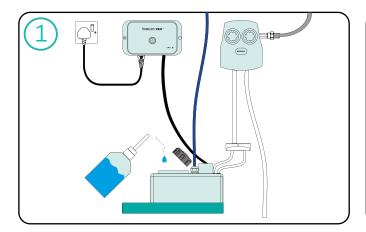
Unscrew the black lid from the empty 5L tank. Add two pumps  $(2 \times 30 \text{ml})$  from the brine solution container. There shouldn't be any water in the tank at this stage.
