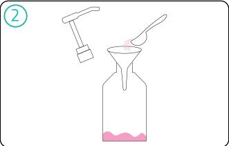
If the salt in the brine bottle has dissolved or the water level is low simply add more salt (to around 5cm level) or water. As long as you can see the salt in the bottom of the water this means it's supersaturated and the correct measure is used.
