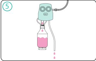
When the solution is activated the unit will beep and the blue light returns to green. The solution is now ready to dispense. The dispensers are set to deliver 20L at 200ppm via the bottle dispenser and 40L at 100ppm via the hose dispenser.
