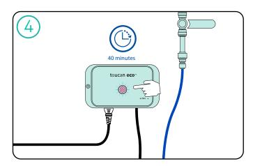
Switch on the activator unit; the switch is on the underside of the unit. The unit's light button will show green. To activate press the green light button. It will turn blue and the activation process starts, which takes 40 minutes.
