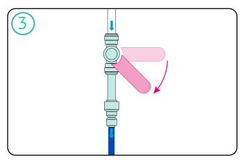
Open the lever valve to fill the tank up to the 5L mark.
