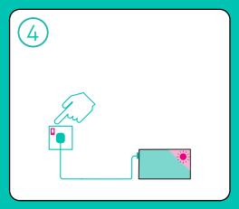
Connect the adapter to the base unit, plug into a wall socket and turn the power on at the wall. The base will beep and lights flash twice.
