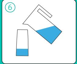
After 5 minutes the base beeps, blue jug and white button lights stay on, and solution stops bubbling. It's now ready to use and pour into the bottle. After 3 minutes you can activate again, indicated by a beep and lights switching off. This prevents the device from overheating.
