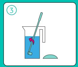
Stir the solution at least 8 times in the centre of the jug to fully dissolve the salt. The salt acts as an electrolyte and if it accumulates on the electrode the product will not work. Place the lid on the jug, and wipe any water away from the electrodes on the bottom of the jug.
