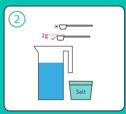
Add 2g of table salt - that's a flat measure using the measuring spoon provided. No more or less as this affects the electrolysis. If too much salt is added, rinse out the jug and start again. Do not use rock salt.
