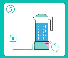
Place the jug on its base. The base will beep once and white button remains lit. Activate the solution by pressing the button once. The base light will flash and beep, the jug will light up blue and bubbles appear as electrolysis begins.
