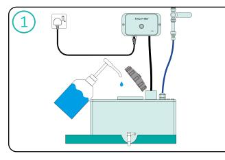
Undo the tank's black lid and add one pump (30ml) of the brine solution. Do not add more as this may prevent the device from activating.
