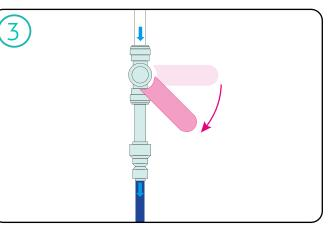
Open the lever valve to fill the tank up to the 10 litre mark. If the unit isn't plumbed in simply fill by hand.
