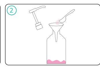
If the salt in the brine bottle has dissolved or the water level is low simply add more salt or water. As long as you can see the salt in the bottom of the water this means it's super saturated and the correct measure is used.
