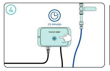
Switch on the activator unit - the unit's light will turn green. Press the button, the light turns blue and the electrochemical activation begins. This will take 15 minutes.
